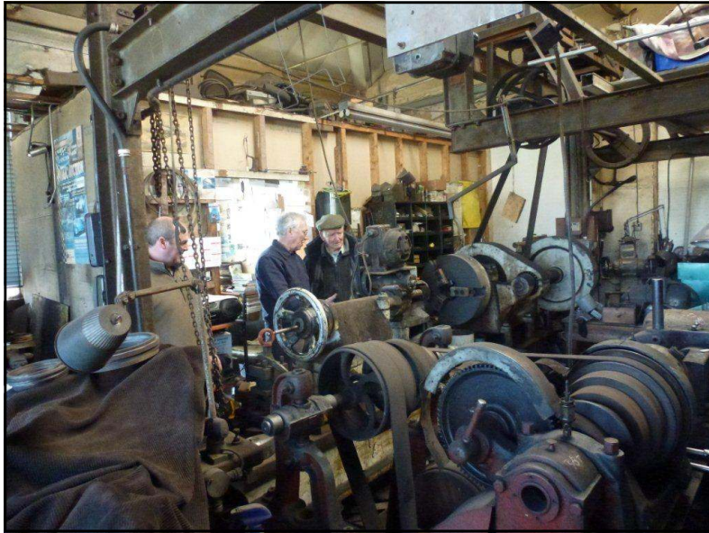
Alan's factory with flat belts driving lathes and machines
